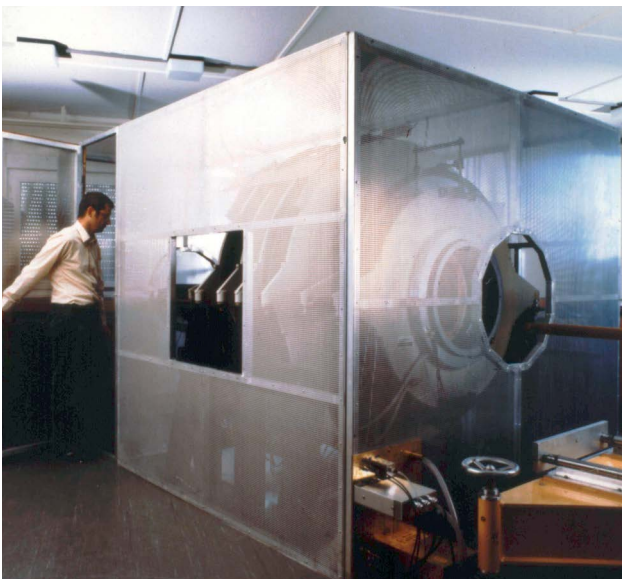
5 RF Faraday cage built around the 0.1T magnet.
