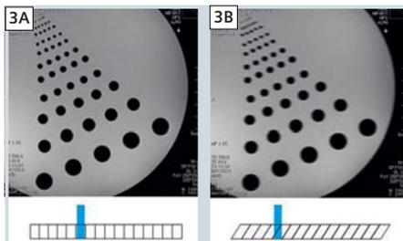
3 VAT\* blurring caused by the shearing of the slice: (3A) Image without VAT: the signal of a vertical structure (vertical blue line) is well localized in a pixel (horizontal blue line); (3B) blurred image with VAT: The vertical structure appears smeared over multiple pixels.
