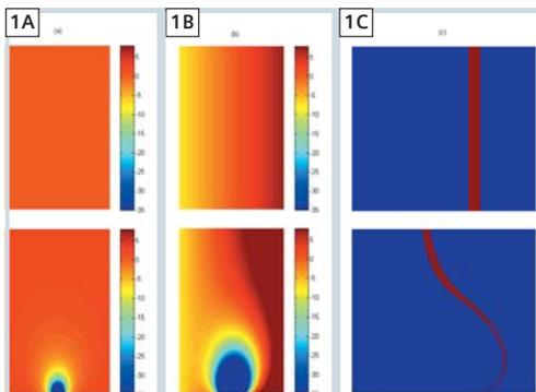
**1** The upper row visualizes the ideal case of slice selection, while the lower row displays the effects on the slice selection by a distorted background field: **(1A)**  $B_0$  field map in slice select direction, **(1B)**  $B_0$  field map in direction of slice encoding with superimposed magnetic gradient field for excitation, and **(1C)** position of the excited slice.
